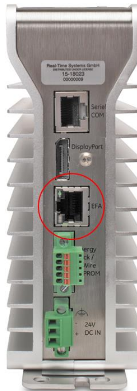
Figure 8: EFA Port on Underside of CPE400 Unit
