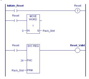
**Note:** It is important to invoke SVC\_REQ #24 for only one sweep at a time. Each time this function executes, the target Ethernet Interface will be reset regardless of whether it has finished starting up from a previous reset. If multiple reset requests (for example, push button to reset Ethernet) occur simultaneously, Ethernet daughterboard will be reset only once rather than multiple times.
