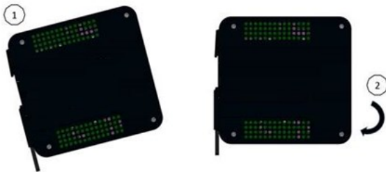
Figure 6: Mounting of the CPE115 on DIN rail
