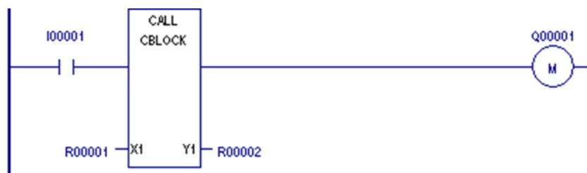
Figure 6: Invoking a C block from Ladder Program
