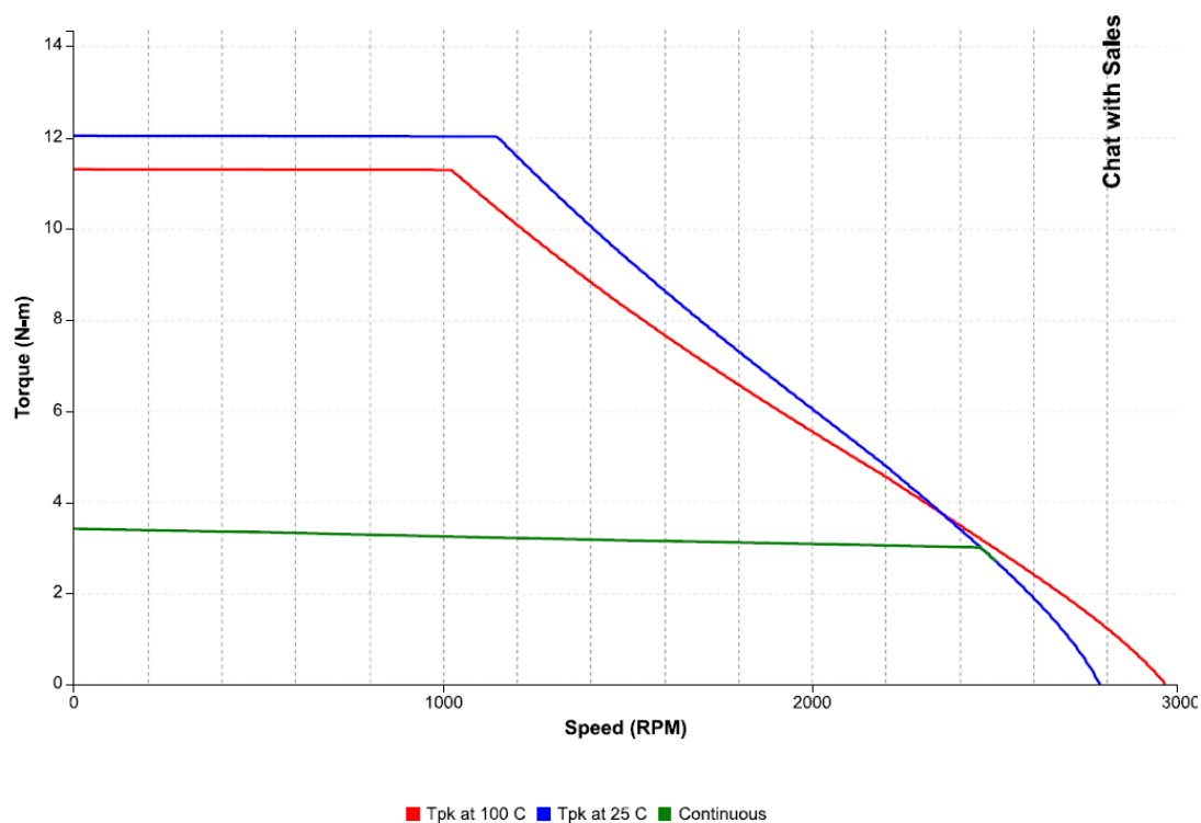
Figure 29: Speed-torque performance of an IC830M42E motor with an IC830DP00606 drive at 230 VAC
