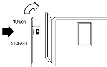
If Run/Stop mode switch operation is enabled, the switch can be used to place the CPU in Run mode.
