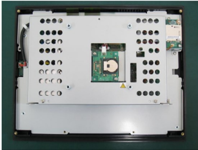
Figure 72: Coin Battery Location IC755CxSxxCDx
