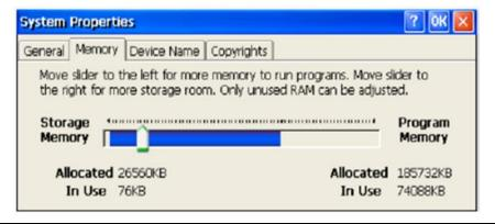
**Note:** Storage memory is limited to a maximum of 128 MB. Using the slide bar to increase storage memory will provide more RAM-based storage in the folder \Object Store.
