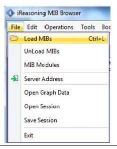
If there are no errors, the MIB will be loaded successfully and the SNMP Manager will be ready for communication with QuickPanel<sup>+</sup> device operating as an SNMP Agent.
