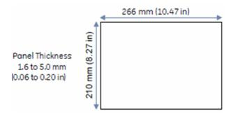
Figure 57: Panel Cutout Dimensions IC755CxS12CDx
