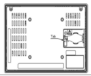
5. Slide the battery cover into place, taking care not to pinch the harness connector.
