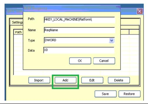
The entered data can be edited by selecting the record in the list box and clicking on the Edit button. This opens the dialog box that allows the user to edit the data.
