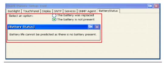
5. If the option **the battery was replaced** is selected, enter the date of when the battery was first used in a QuickPanel<sup>+</sup> device. (This date should reflect the date of first use in any QuickPanel<sup>+</sup> device, not just the current device.)
