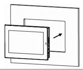
4. Insert the hook of the mounting bracket into the mounting hole as displayed in the following figure.
