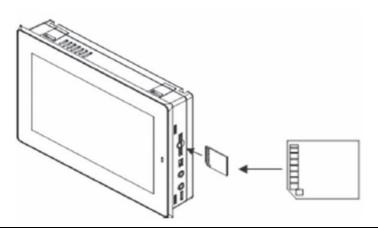
Figure 80: SD Card Location IC755CxW07CDx
