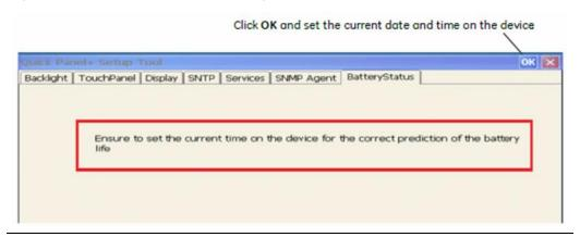
2. After setting the current time, open the QuickPanel<sup>+</sup> Setup Tool, and select the **BatteryStatus** tab to display the correct battery life prediction information.
