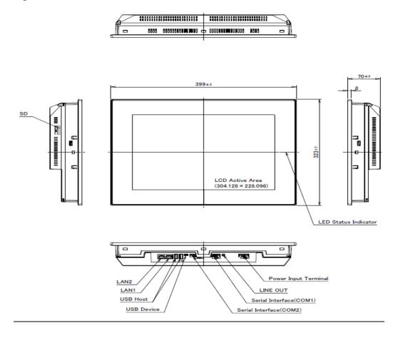
Figure 11: Rear View IC755CxS15CDx
