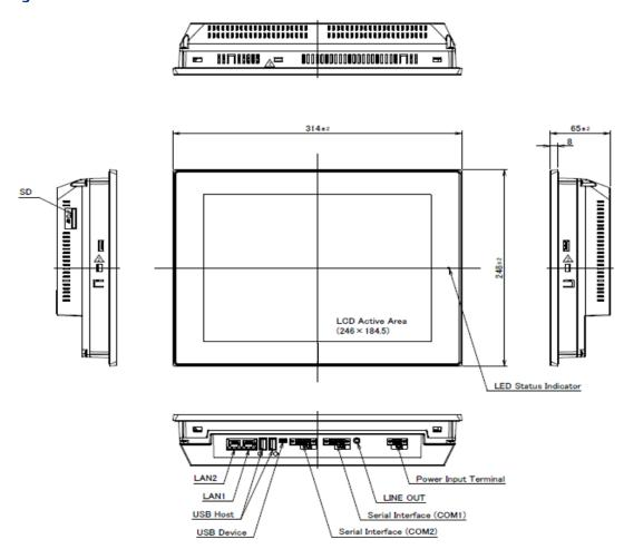
Figure 9: Rear View IC755CxS12CDx
