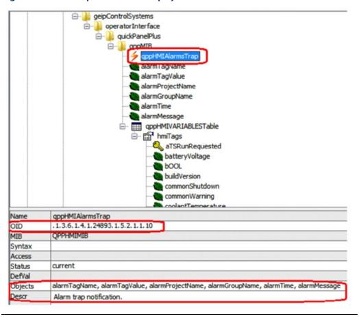
Figure 39 displays the list of HMI Tags that the SNMP Manager can query to retrieve live values from the HMI running on a QuickPanel<sup>+</sup> device.
