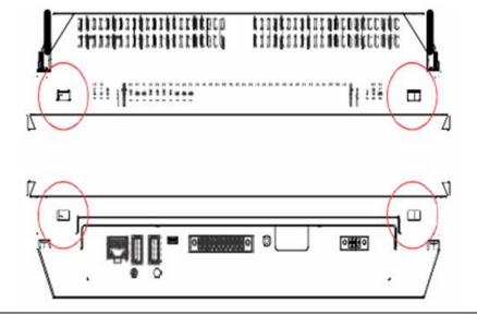
The IC755CxS12CDx and IC755CxS15CDx mounting holes are located on the top, bottom, and sides of the unit.
