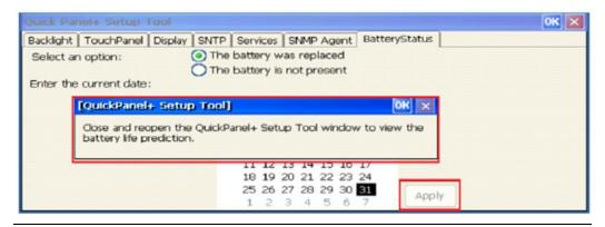
Figure 35: Battery Life Prediction Example after Battery Replacement
