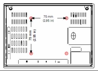
Figure 63: VESA Mounting Holes IC755CxSxxCDx
