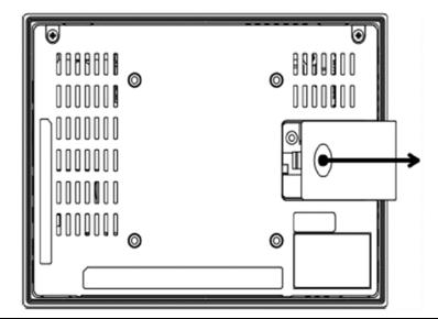
2. Connect the battery harness connector to the header, noting keyed orientation.
