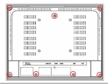
2. Gently press on either side tab to release the back cover.
