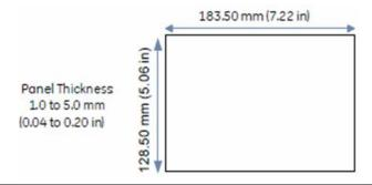
Figure 56: Panel Cutout Dimensions IC755CxS10CDx
