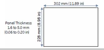
Figure 58: Panel Cutout Dimensions IC755CxS15CDx
