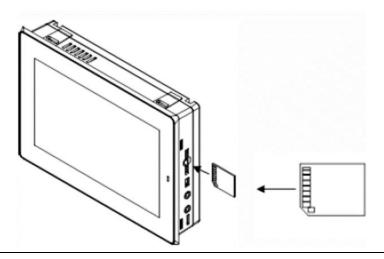
Figure 81: SD Card Location IC755CxSxxCDx
