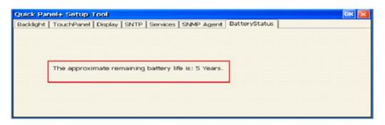
**Note:** If the current time is not set on the device, the QuickPanel<sup>+</sup> Setup Tool dialog box will not be capable of providing an accurate battery life prediction.
