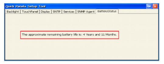
3. If the battery was replaced or removed on the QuickPanel<sup>+</sup>, QuickPanel<sup>+</sup> Setup Tool **BatteryStatus** displays two possible scenarios related to the battery. (The battery life prediction is estimated based on this selection.)
