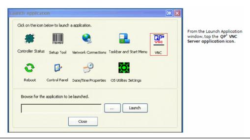
**Note:** The VNC server starts approximately 40 seconds after the QuickPanel<sup>+</sup> start-up process has completed.
