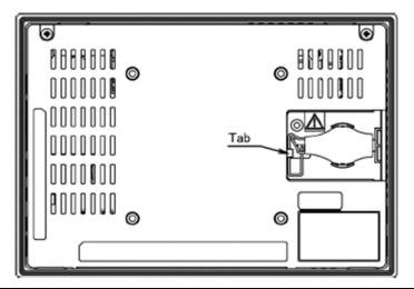
5. Slide the battery cover into place, taking care not to pinch the harness connector.
