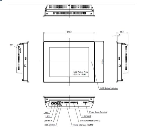
Figure 7: Rear View IC755CxS10CDx
