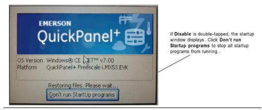
If Use DIP Switch checkbox has been selected, **don't run Startup Programs** displays on the startup window based on the position of DIP Switch 2.
