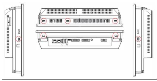
Figure 54: Mounting Holes (all four edges) IC755CxS15CDx
