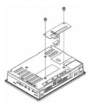
2. Connect the USB cable and insert the retaining clamp into the retaining clamp plate.
