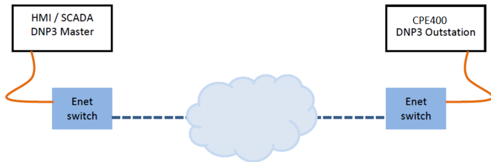
Figure 1: DNP3 Basic System Architecture
