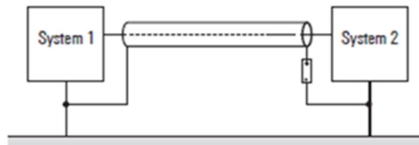
Figure 308: Shield Grounding at Both Ends with High-Impedance at One End
