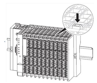
2. Swivel the plug-in unit with the cabling towards the front by 90°.
