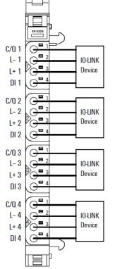
The EP-5324 module is an IO-Link master according to the IO-Link specification V1.1.2. One IO-Link device can be connected to each connector. The IO-Link devices must conform to port class A. Port class B is also possible if additionally, potential distribution modules are used. One digital input can be used additionally with each connector.
