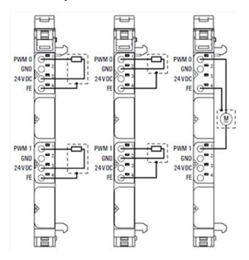
The digital pulse width modulation modules EP-5442 is used for the control of small motors with current requirements of up to 2 A. The period duration for each channel can be parameterized from  $25\mu$ s to
