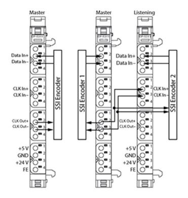
The EP-5311 SSI Encoder Interface module can read differential signals (RS422) from a SSI encoder. It can be connected as a master directly to the encoder providing the clock. To synchronize two SSI encoders a second SSI module running in Listening mode can be placed between the encoder and a master module from which it receives the clock.
