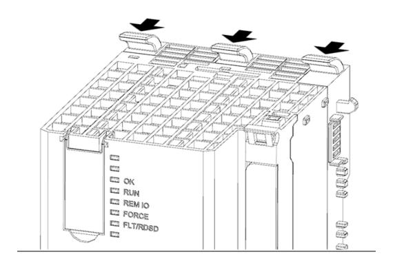
2. Attach the controller to the DIN rail. The controller should rest on the rail, but be able to move freely side-to-side.
