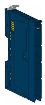
Empty slot modules can be integrated as reserve modules in a station. They bridge all contacts in the basic module 1:1 and otherwise have no function. Empty slot modules are passive modules without fieldbus communication, therefore they are not considered during configuration.
