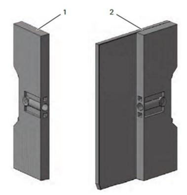
Each RSTI-EP fieldbus network adapter is delivered together with a termination kit EP-8301. This comprises two end brackets and an end plate. The end plate protects the contacts on the last module at the end of the RSTI-EP station. The station is fixed to the DIN rail on both sides via the end brackets.
