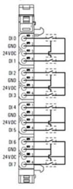
The digital input module EP-1318 can detect up to 8 input signals. Two sensors can be connected to each connector using a 2-wire or 3-wire connection. A status LED is assigned to each channel. The module electronics supply the connected sensors with power from the input current path (IIN).
