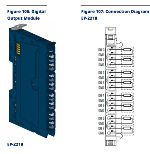
The EP-2218 digital output module can control up to 8 discrete outputs, each with a maximum of 0.5A. Discrete outputs can be connected to each connector in a 2-wire connection. A status LED is assigned to each channel. The outputs are supplied with power from the output current path (IOUT).
