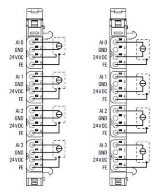
left: 3-/4-wire sensor with sensor wiring via electronics.
