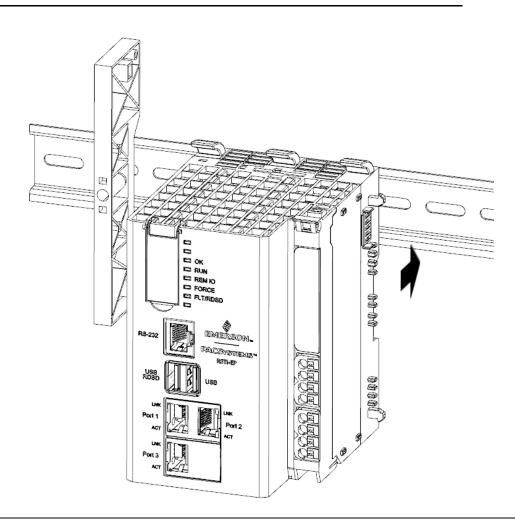
1. Slide the controller along the DIN rail into place. The controller should be in the leftmost position and rest against a stop block (if applicable).
