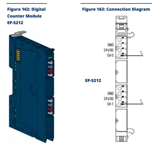
The digital counter module EP-5212 can read frequency of one squarewave signal (1 channel) from one or two external sensors with a maximum input frequency of 100 kHz. Frequencies to be counted are applied to channel CH0 and/or channel CH1, the measurement will be started via control word 1 and 2 respectively. Measuring cycles can be defined in  $\mu$ s. The longer the measuring cycle the more exactly the measurement.
