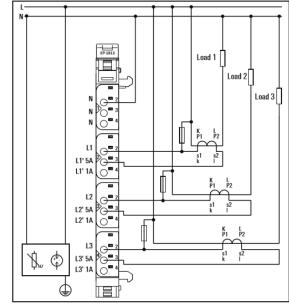
**Note:** If the module is used in an environment of overvoltage category III, transient overvoltage must be limited to  $\leq 2500V$
