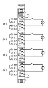
The digital input module EP-1804 can detect up to 4 binary control signals. One sensor can be connected to each connector using a 2-wire connection. Both L and N connections of each input are bridged internally. The four inputs are galvanic isolated, they can be supplied with input voltages between 110Vac and 230Vac. Solely AC measurements can be run.
