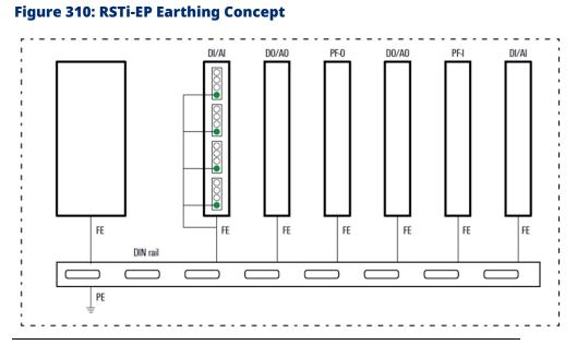
The spring contacts underneath the module and the network adapter snap into the DIN rail to make a connection.
