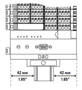
A RSTi-EP station may only be installed in this sequence (starting from the left/bottom):
