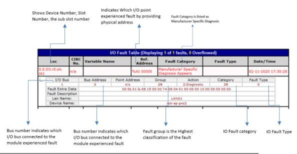
As shown in Figure 36, 17 bytes of Fault Extra Data is provided in IO Fault table as a part of Vendor Specific Diagnostic Data.<sup>3</sup>
