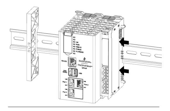
2. Repeat the steps for each of the IO modules. Connect the first IO module into connectors on the right side of the controller. Each subsequent IO module will connect to the previous module.
