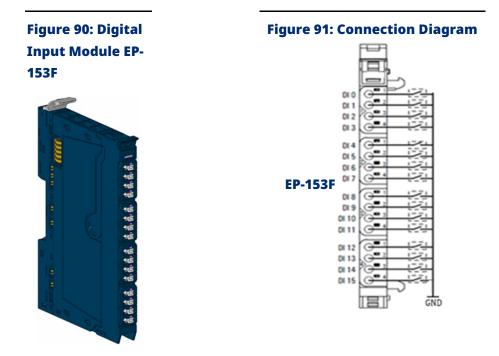
The EP-153F digital input module can detect up to 16 input signals. Four sensors can be connected to each connector in a 1-wire connection. A status LED is assigned to each channel. The connected sensors must be supplied with power from the input current path IIN (e.g. with potential distribution modules).
