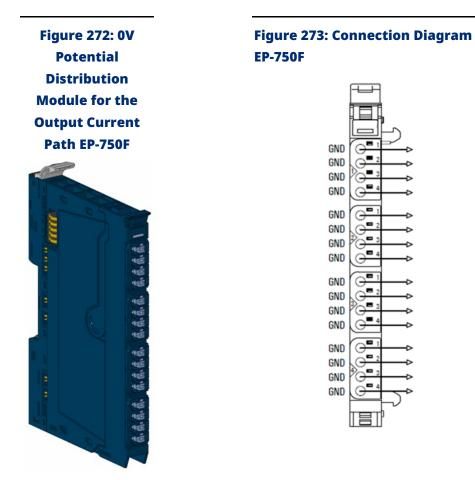
The potential distribution module EP-750F provides 16 connections for ground from the output current path. Potential distribution modules are passive modules without fieldbus communication, therefore they are not considered during configuration.
