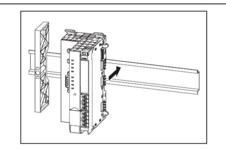
6. Slide the bus network adapter to the left until it completely connects with the end bracket. At the same time, press the bus network adapter as close as possible to the DIN rail so that the network adapter is not tilted.
