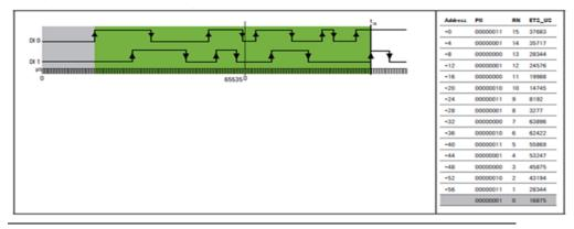
A falling 1-0 edge on DI 1 causes the17th ETS entry. The 2nd ETS entry is deleted and not available anymore.
