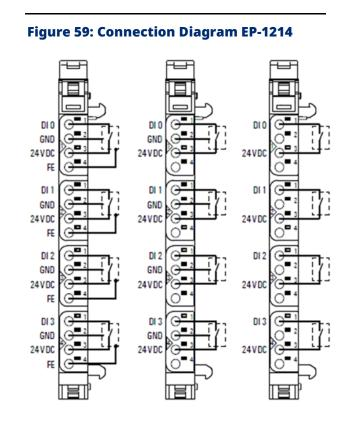
The digital input module EP-1214 can detect up to 4 input signals. One sensor can be connected to each connector using a 2-wire, 3-wire or 3wire + FE connection. A status LED is assigned to each channel. The module electronics supply the connected sensors with power from the input current path (IIN).
