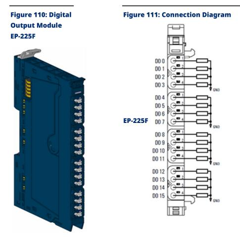
The EP-225F digital output module can control up to 16 discrete outputs, each with a maximum of 0.5 A. Four discrete outputs can be connected to each connector. A status LED is assigned to each channel. The outputs are supplied with power from the output current path (IOUT).
