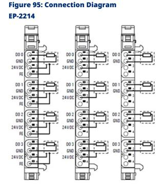
The EP-2214 digital output module can control up to 4 discrete outputs, each with a maximum of 0.5 A. One discrete output can be connected to each connector using a 2-wire, 3-wire or 3-wire connection + FE. A status LED is assigned to each channel. The outputs are supplied with power from the output current path (IOUT).
