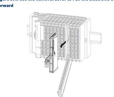
Figure 396: Use the Removal Lever to Pull the Electronic Unit **Forward**
