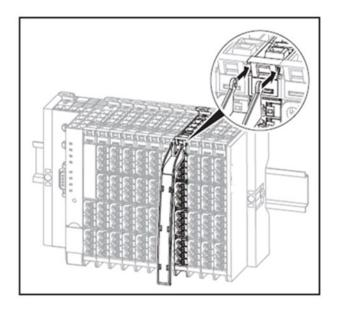
16. Insert the labelled marker into the swivel marker from below.
