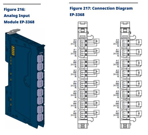
The analog input module EP-3368 can detect up to 8 analog sensors with 0-20 mA or 4-20 mA. The resolution is 16 bits per channel. Sensors can be connected to each connector in a 2-wire, 3-wire or 3-wire connection + FE (IDC). The measurement range is defined using parameterization. A status LED is assigned to each channel. The module electronics supply the connected sensors with power from the input current path (IIN).
