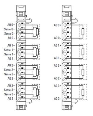
The analog output module EP-4264 can control up to four analog actuators with  $\pm 10$  V,  $\pm 5$  V, 0-10 V, 0-5 V, 2-10 V, 1-5 V, 0-20 mA or 4-20 mA. The resolution is 16 bits per channel. An output can be connected to each connector, the internal switching is carried out automatically. The output range is defined using parameterization. A status LED is assigned to each channel. The outputs are supplied with power from the output current path (IOUT).
