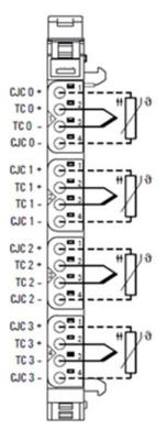
The analog input module EP-3804 can detect up to 4 analog thermocouple sensors or voltages between ±15 mV and ±2V. The resolution is 16 bits per channel. Sensor type and temperature range are set using parameterization. Mixed operation using different sensors is possible. For each channel, an internal or external cold-junction compensation (CJC) can be parameterized. A status LED is assigned to each channel.
