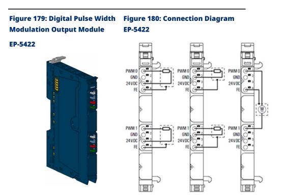
The digital pulse width modulation module EP-5422 is used for the control of small motors with current requirements of up to 0.5 A. The period duration for each channel can be parameterized from  $25\mu$ s to approx. 175ms (input values from 1,202 to 8,388,607 based on a factor 0.02083 $\mu$ s).
