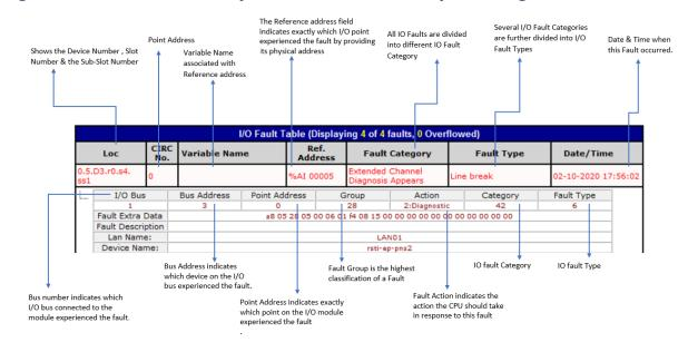
As shown in Figure 33, 21 bytes of Fault Extra Data is provided in IO Fault table as a part of Extended Channel Diagnostic Data.
