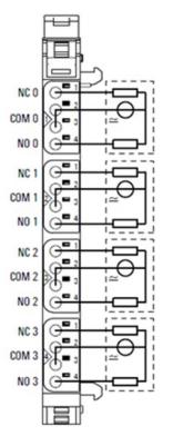
The digital relay output module EP-2714 can control up to 4 discrete outputs, each with a maximum of 6A. Each connector features a potential-free changeover contact. The relay coils are supplied with power from the output current path ( $I_{OUT}$ ).
