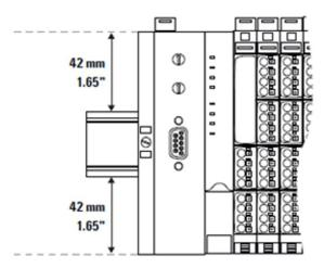
Installation on vertically positioned DIN rails is also possible. In this case however, the heat dissipation is reduced such that the derating values change (refer to Section 3.5, Current Demand and Power Supply). In the case of vertical mounting, the network adapter must always be arranged as the first module at the bottom and secured with an end bracket for vertical mounting.
