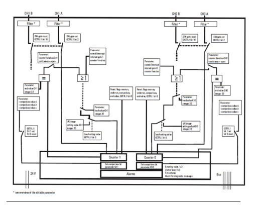
Figure 160: EP-5112 Counter Operation Using Rotary Transducer
