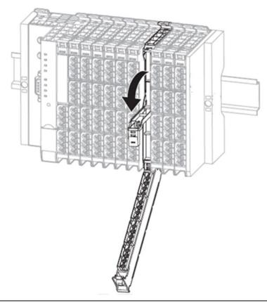
3. Using the removal lever, pull the electronic unit forwards and out.
