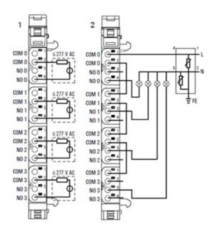
The solid-state relay output module EP-2814 uses four semiconductor switches to control up to 4 discrete outputs, each with a maximum of 1A at 255Vac. The switching characteristics of the semiconductor switch have it as being closed when the voltage crosses zero and open when the current crosses zero. Each connector features a potential-free NO (Normally Open) contact.
