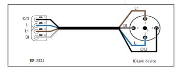
**Note:** The use of the additional digital input at the DI connection is optional. It can be use as digital input, e.g. if the IO-Link device provides an additional switching signal.
