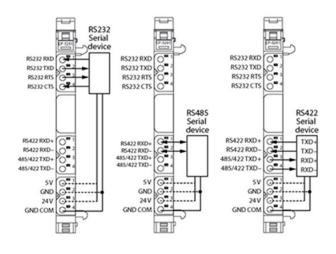
Serial data can be exchanged between the PLC and a data terminal device using the EP-5261 communication module. The device (such as a barcode scanner, printer) can be connected through an interface type RS232, RS485 or RS422.
