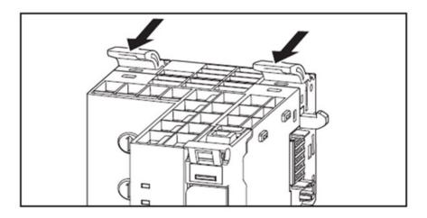
5. Place the field bus network adapter (module side to the right) on the DIN rail so that it audibly clicks into place.
