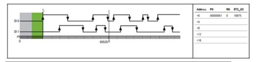
A rising 0-1 edge on DI 1 causes the 2nd ETS entry at address + 0. The 1st ETS entry is shifted by 4 bytes.
