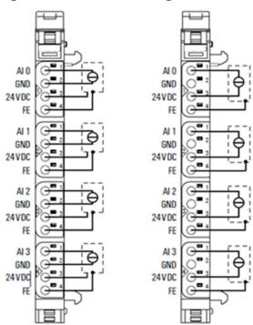
Left: 3-/4-wire sensor with sensor wiring via electronics
