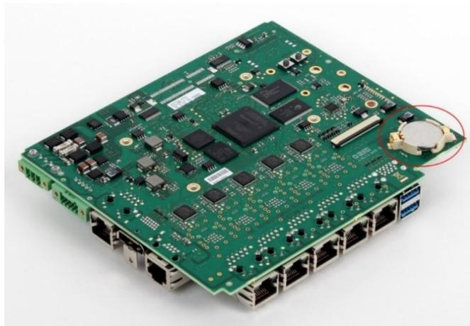
The CPE400/CPL410 is shipped with a real-time clock (RTC) battery installed on an internal circuit board (Figure 6). This battery will need to be replaced periodically by a qualified service technician. Typically, no action is required during initial installation.
