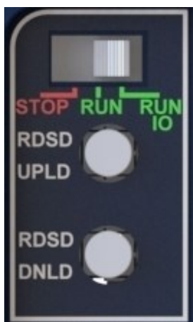
Figure 10: CPE330 Run/Stop Switch and RDS Switches
