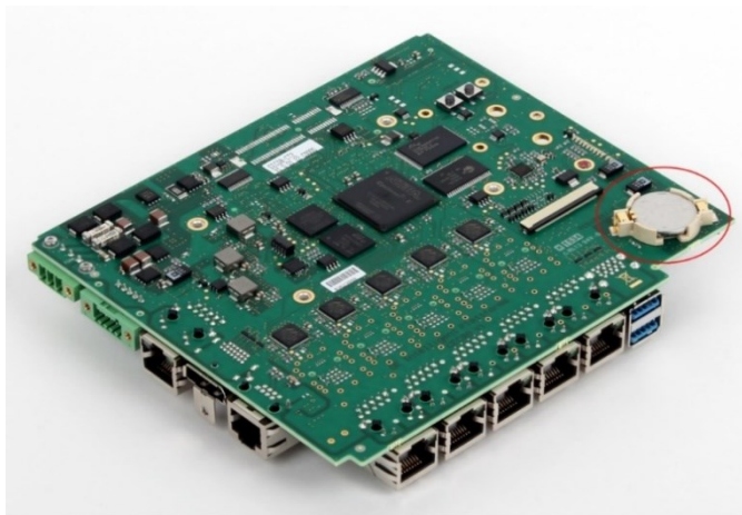
Figure 19: Location of RTC Battery on CPE400
