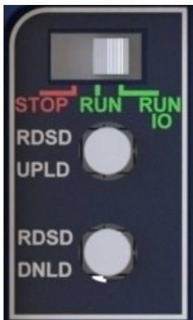
Figure 23: CPE330 Run/Stop Switch and RDSD Switches
