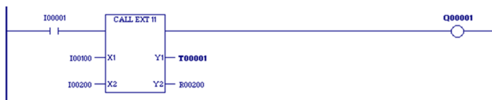
Figure 8: Calling an External Block in Ladder Logic
