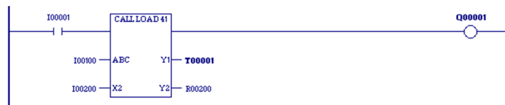
Figure 3 Block Call with Parameters
