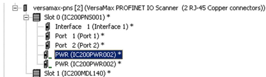
Adding power supplies to the configuration sets up power supply alarms. Alarms will be triggered if the power supply is configured but not working or configured in the wrong subslot. These power supplies have no configurable parameters, but their power supply and GSDML details can be viewed by double-clicking on a power supply icon or right-clicking and selecting Configure.
