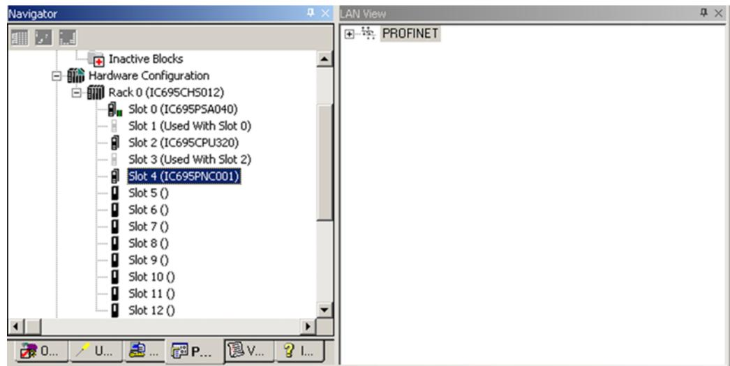
Adding a PROFINET Controller to the project automatically creates a new LAN.
