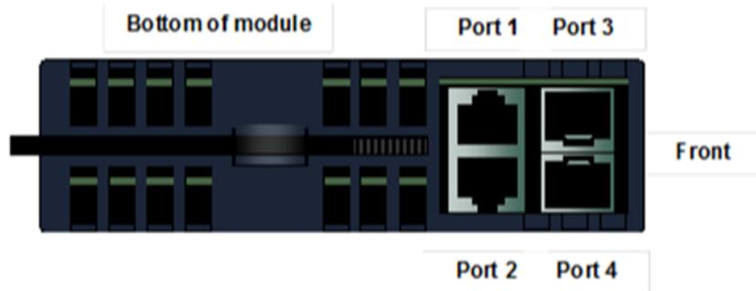
For the Embedded PROFINET LAN (LAN2), CPL410, CPE400 and CPE330 both provide two RJ45 ports identical to those shown as Port 1 and Port 2 in Figure 4. The operational behavior, configuration parameters and diagnostics are also identical. Refer to the corresponding product documentation for further details.
