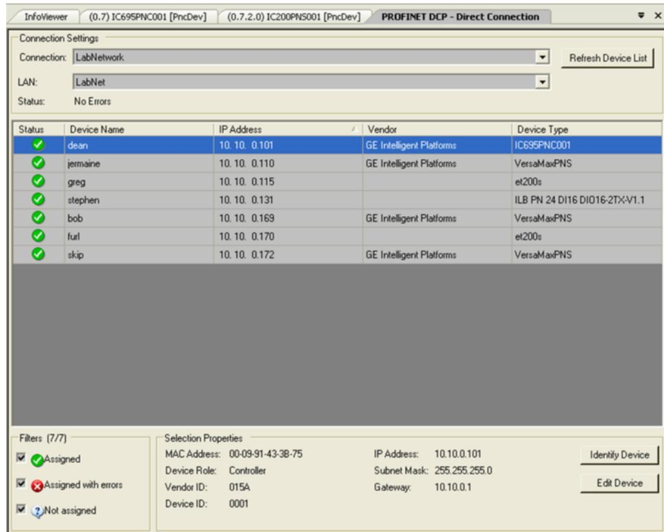
If the Device Name of the device on the network is not correct, select the target device in the list of networked devices, and click Edit Device. This will open a new dialog that can be used to set various parameters, including Device Name, directly on the device.
