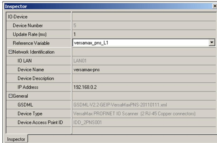
**IO LAN:** (read-only) identifies the LAN of which the IO-Device is a part.
