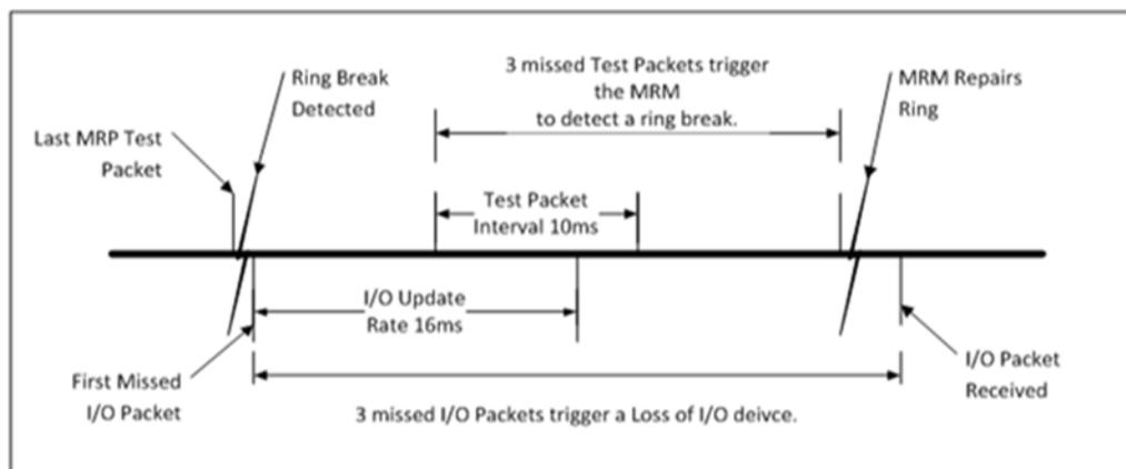
To ensure a successful ring recovery using the Test Packets at a 16ms I/O Update rate or above, make sure the following statement is true:
