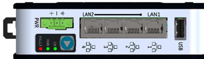
The CPE100/CPE115 Embedded PROFINET LAN (LAN2) supports three switched 8-conductor RJ45 shielded twisted pair 10/100 Mbps copper interfaces ports as shown in Figure 5. The operational behavior, configuration parameters and diagnostics are identical to PROFINET port of CPE400. Refer to the corresponding product documentation for further details.
