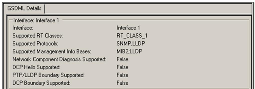
Double-clicking on the PNS module's Port 1 and Port 2 icons in the Navigator also displays additional GSDML parameters for the scanner:
