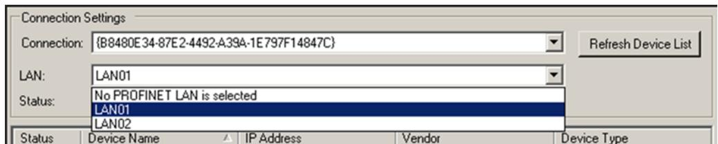
Once a LAN is selected, click on *Refresh Device List* to display a list of actual devices on the LAN. Each device can be in one of three conditions as indicated by the symbol in the *Status* column:
