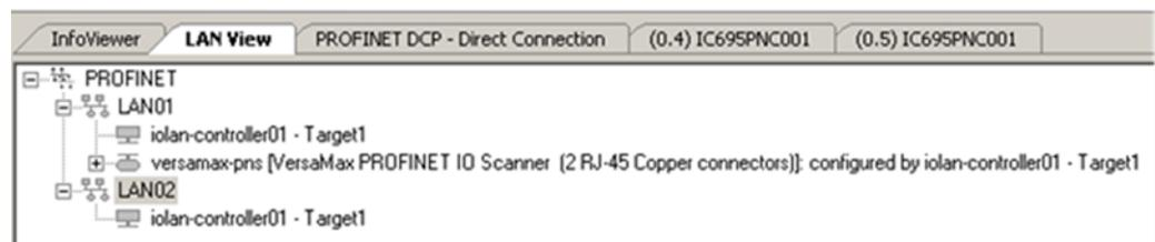
A PROFINET Controller can be moved to a different LAN by selecting the module in the Navigator and dragging it to the target LAN. Here, the PROFINET Controller has been moved from LAN02 (Figure 38) to LAN01 (Figure 39):
