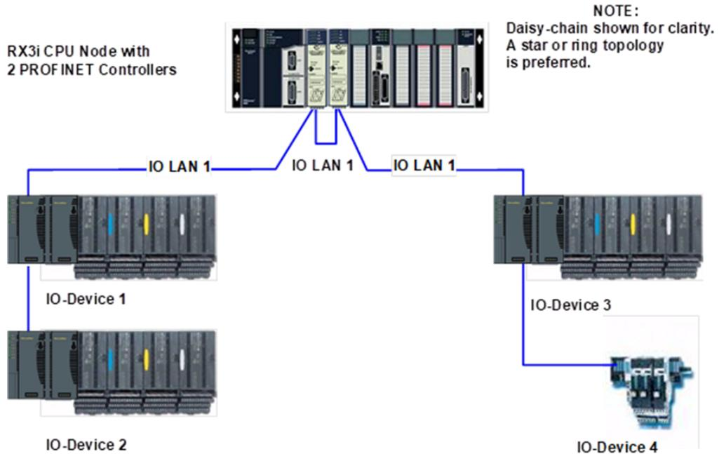
In Figure 10, the two PROFINET Controllers are connected to separate networks. The maximum number of IO-Devices with multiple PROFINET Controllers in the same RX3i controller is 255.
