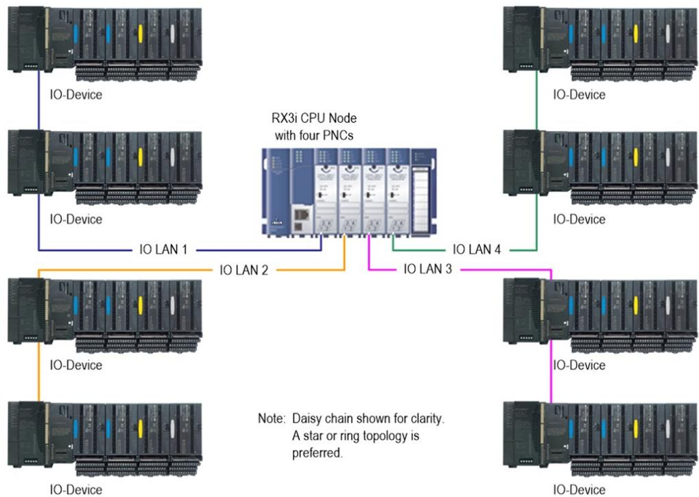
As in the other examples, other Emerson IO-Devices can be substituted for the VersaMax PROFINET Scanners.
