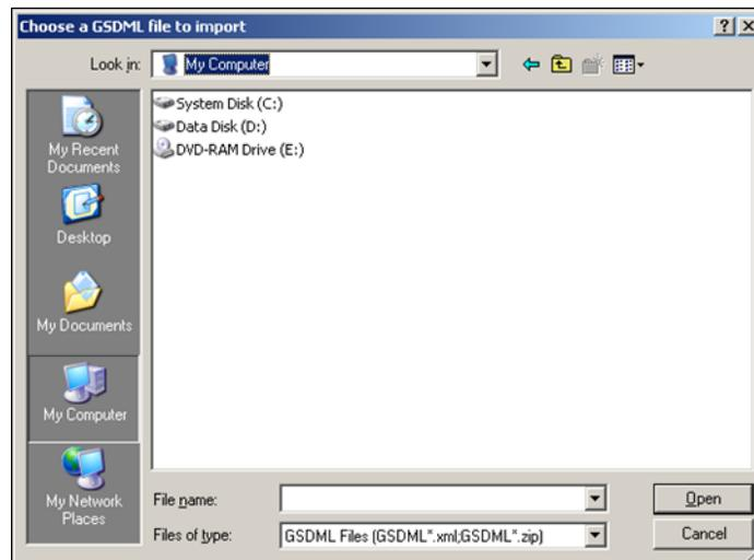
Provide a filename path to the file and click OK. The device is added to the configuration. Machine Edition extracts necessary parameters from the GSDML file and makes the data available for editing within Machine Edition.
