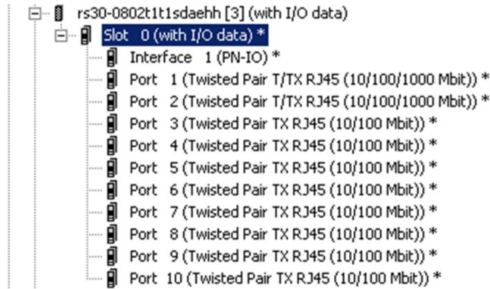
The device in Figure 79 is a switch. The parameters of its ports can be viewed and edited by either double-clicking on a port or selecting a port then right-clicking and selecting Configure from the menu.
