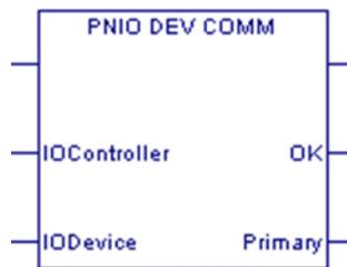
PNIO\_DEV\_COMM can be used by the application logic to take a corrective action or turn on an indicator if a specific device fails. It might also be used by a custom HMI to show which PROFINET IO-Device connections are currently established.
