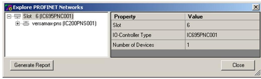
Figure 37: Explore PROFINET Network from Embedded PROFINET Controller
