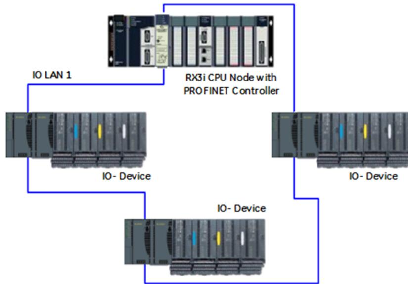
As a Media Redundancy Manager, the PROFINET Controller detects when the network ring has been broken and repaired. Each time the PROFINET Controller detects that the ring has been broken or repaired, a fault is reported in the Local Log table and that condition is passed to the RX3i CPU to be registered in the CPU fault table. In addition, the PROFINET Controller keeps a count of break/repair detections. In the PNC001-Ax module, this may be viewed via the CLI `show rdnmedia` command.
