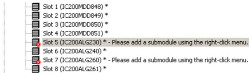
Double-clicking one of these modules, or right-clicking and selecting Configure displays only the Power Consumption and GSDML tabs. The Settings tab and other configuration tabs do not appear. To begin configuring one of these modules, right-click the module in the Navigator and select Change Submodule List from the menu.
