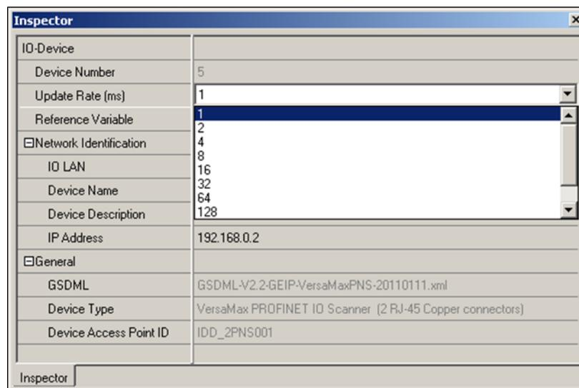
**Note:** Note that shorter update periods place higher processing loads on the associated PROFINET Controller. Refer to above Section, PROFINET Controller Loading Limits. A PNC001 module can handle heavier loads than an equivalent embedded PROFINET Controller.
