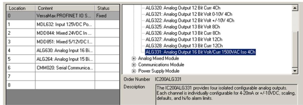
To delete a module from the left-side pane, select it and press the keyboard Delete key. When the modules in the left side pane are correctly situated, click OK to add them to the Configuration.
