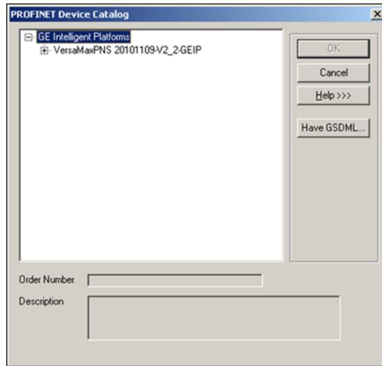
In the PROFINET Device Catalog, expand the VersaMax PNS line and choose the module type:
