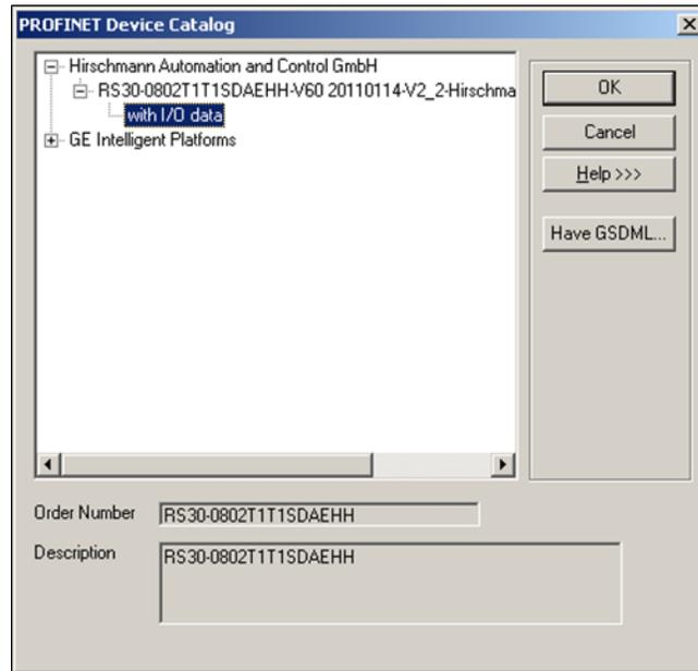
To be included in the system configuration, any third-party IO-Device requires a GSDML file. The GSDML file for the device must be present on the computer being used for the configuration.
