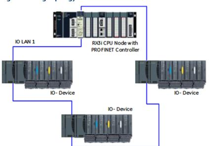
Figure 99: Ring Topology with One Controller
