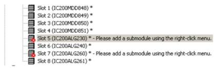
Double-clicking one of these modules, or right-clicking and selecting Configure displays only the Power Consumption and GSDML tabs. The Settings tab and other configuration tabs do not appear. To begin configuring one of these modules, right-click the module in the Navigator and select Change Submodule List from the menu.
