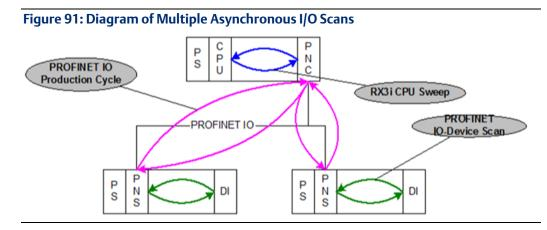
PROFINET IO-Device Scan: in Figure 91, each VersaMax PNS scans all the modules in its node as quickly as possible. The PNS stores the input data gathered from each of the input modules in that node into its internal memory. On each output scan, the PNS writes the output data from its internal memory to the output modules in its node.
