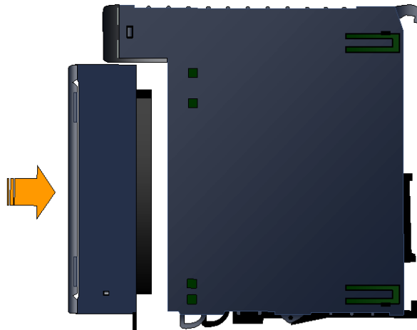
Figure 443: Installing a High-Density Terminal Block
