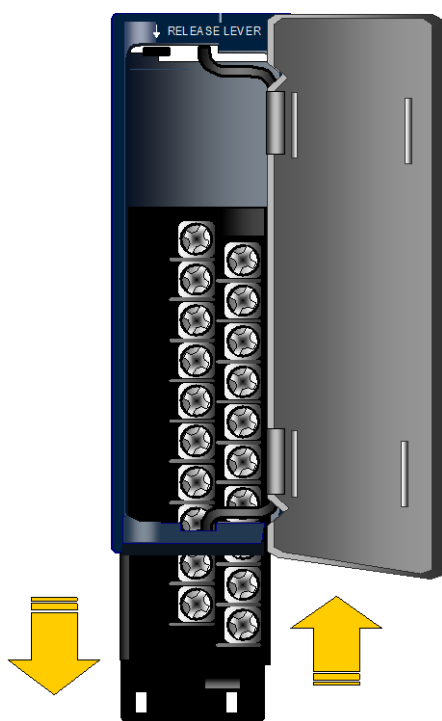
Figure 32: Extraction or Insertion of Terminal Block into its Cover
