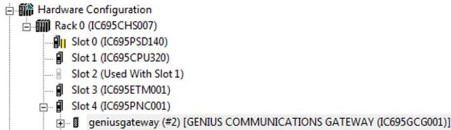
**Note:** Genius gateway... is the default PROFINET Device Name that PME gives to a GCG001 in the Hardware Configuration under a PNC001. This Device Name must match that given to the module itself using the PROFINET/DCP (Discovery and Configuration Protocol) tool (see Figure 12). If there are multiple GCG001s on a PROFINET bus, each of the modules' Device Names must be unique. You can change it by selecting the device in the Navigator, then typing in a new name in the Inspector.
