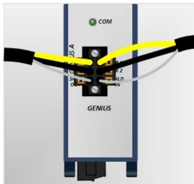
**Figure 11: Genius Bus Wiring for Bus Termination**
