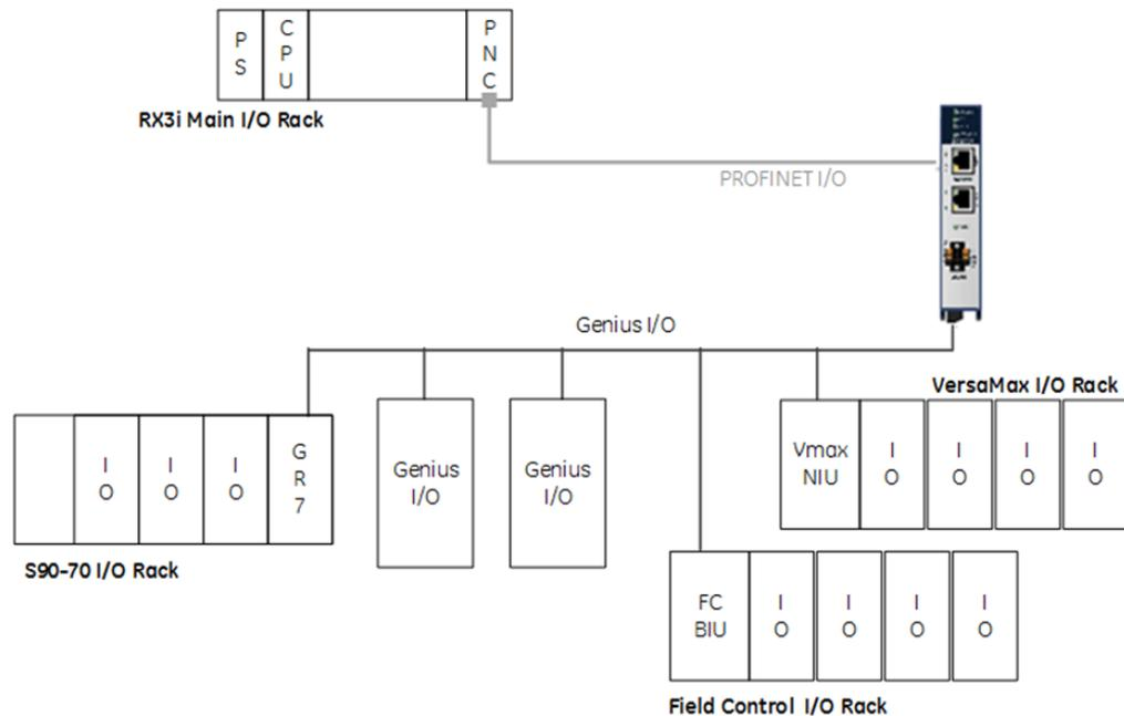
The GCG001 operates as a Genius Bus Controller on a Genius network. It scans the Genius IO devices configured to it, retrieving input data and providing output data. It then exchanges that data with its configured PROFINET IO Controller over its Ethernet interfaces at the configured production rate. The GCG001 can manage communications for up to 31 Genius IO devices on a single Genius Serial Bus.
