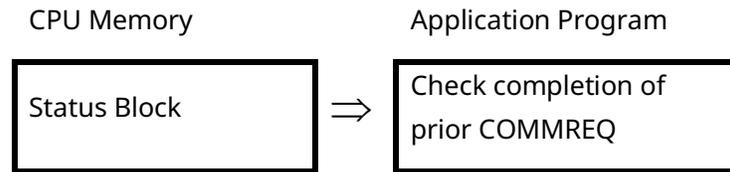
When the previous COMMREQ has completed, the user's PLC program should set the Status Block to zero. Establishing this initial condition allows the program to differentiate between the result of an earlier command and the currently-executing command.
