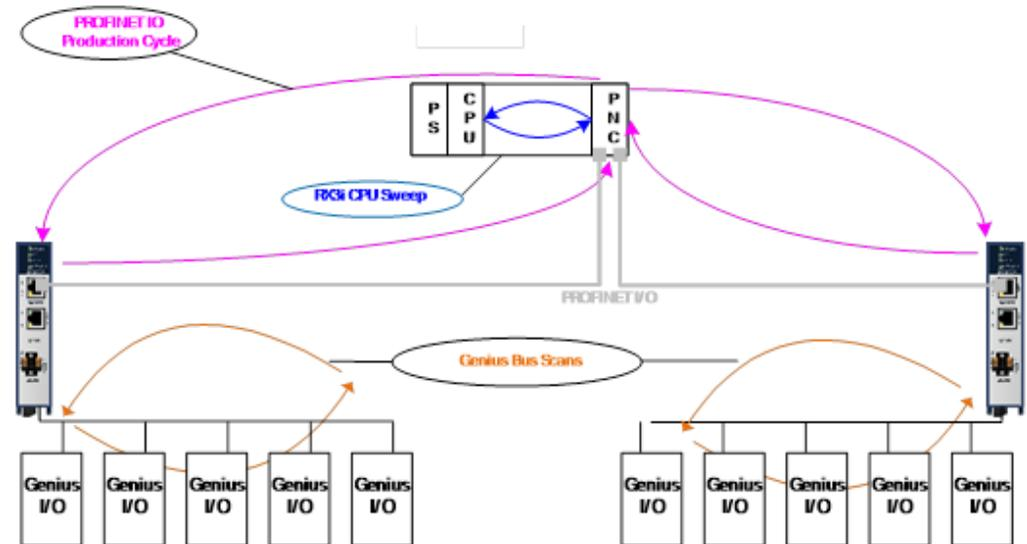
**Genius IO-Device Scan:** In this example, each GCG scans all its Genius devices. The GCG stores the devices' input data into its internal memory. Every time the GCG gets a turn on the Genius bus, it transmits the output data from its internal memory to each of the Genius devices.
