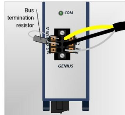
Two terminals each are provided on a removable terminal block for Serial 1, Serial 2, and Shield connections. The figure (above left) shows the Genius connection continuing through the connector block (daisy chain).
