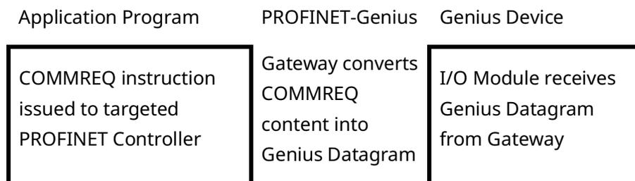
4. Check the status of the initiated COMMREQ task. COMMREQs should be executed sequentially. The application program should check that the status of the previous COMMREQ to the targeted PROFINET Controller is complete before sending it another one. Failure to do this may result in improper operation of the PROFINET Controller.
