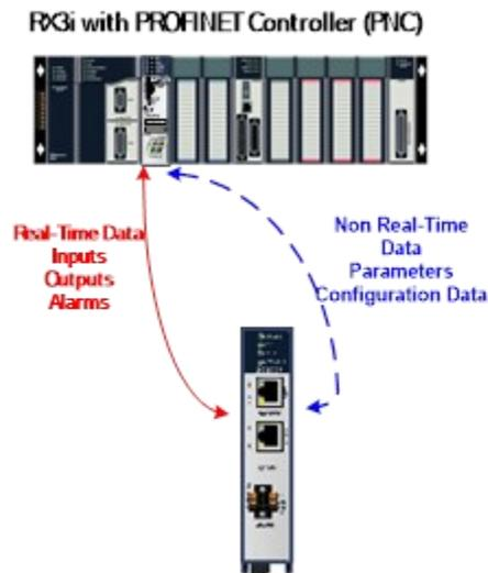
Real-Time (RT) communication: PROFINET real-time communication is used for time-sensitive data. A PROFINET IO-Controller (PROFINET Controller) and PROFINET IO-Device use two types of real-time communications to exchange data: cyclic communication and acyclic communication:
