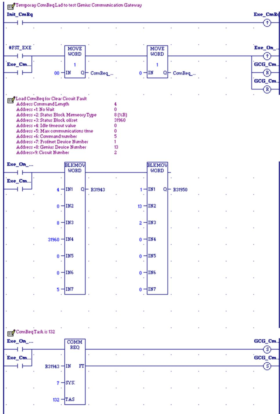
Figure 37: Data\_Init\_Comm to Clear Circuit Fault
