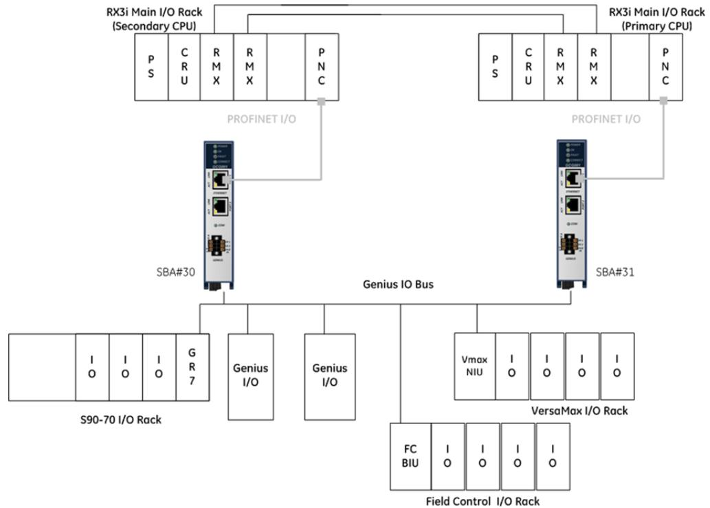
To support either Genius Hot Standby or Duplex type redundancy, two GCG001 modules are present on the same physical Genius Bus, one at SBA #31 and the other at SBA #30, as shown Figure 27. This architecture is designed to withstand the loss of one GCG001 and/or the loss of the PLC to which it is attached. The two GCG001 modules involved should therefore be powered via independent 24Vdc power supplies. Alternately, a Genius Bus Controller may be used at SBA #30 or #31.
