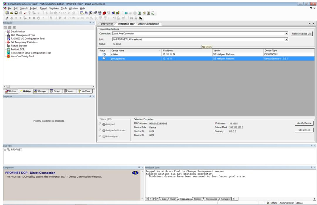
Initially, the out-of-the box GCG001 will not have a name assigned. Select the row containing the GCG001, then click on the Edit Device button in order to assign a unique name.
