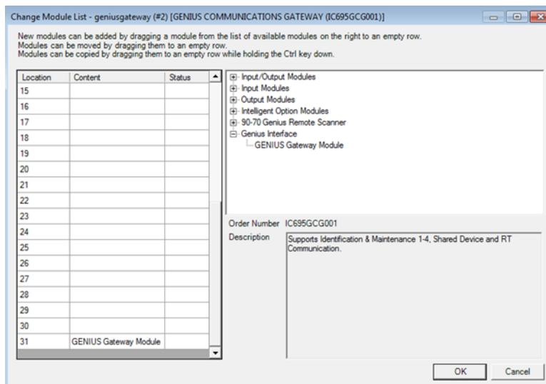
12. Select individual Genius I/O devices from the right-hand panel of Figure 17 and then drag/drop them into the appropriate location row on the left-hand side, resulting in Figure 18.
