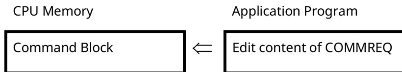
2. Clear status block. The program should set the status block to all zeroes (see programming example Figure 36). Establishing this initial condition allows the program to differentiate between the result of an earlier command and the currently-executing COMMREQ command.
