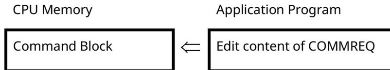
Data is placed in adjacent locations in CPU memory to form a Command Block, per the format shown below:
