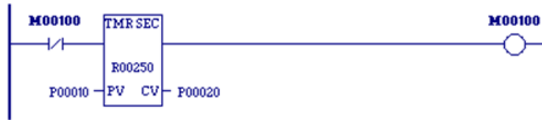
Figure 43: Ladder Logic for Synchronizing Timer
