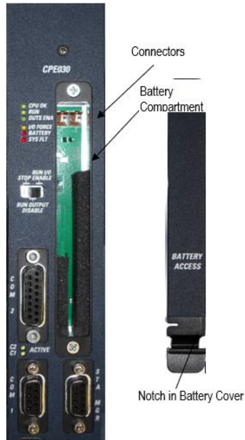
Figure 6: RX7i Battery Installation
