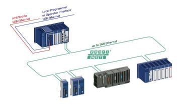
A typical application will take advantage of the two independent LANs. The dedicated LAN1 port will be used for communications with plant-level or supervisory layers. The switched LAN2 will typically be used to communicate with devices within the manufacturing cell or process, including local HMI devices and micro-controllers.
