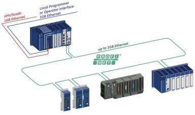
A typical application will take advantage of the two independent LANs. The dedicated LAN1 port will be used for communications with plant-level or supervisory layers. The
