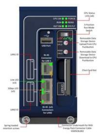
support for up to 32 I/O devices and update rates of 1 – 512ms. I/O device update rates of 8ms and faster are possible with 16 or fewer devices. When there are more than 16 devices configured, update rates of 16ms and higher are available.
