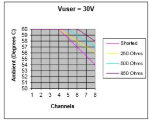
Figure 2: Thermal Derating Charts ALG728 in Current Mode
