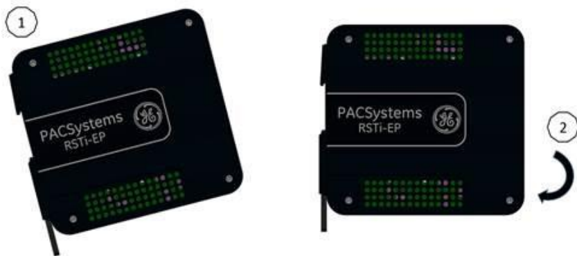
Figure 5: Mounting of the CPE100 on DIN rail
