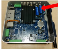
Figure 14: Supercapacitor Board Location
