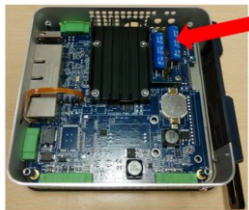
Figure 14: Supercapacitor Board Location
