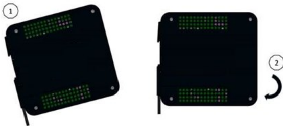
Figure 6: Mounting of the CPE100 on DIN rail
