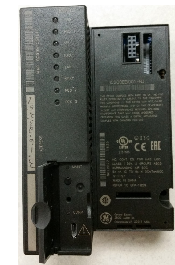
Figure 1: IC200EBI001-MH or later (New Hardware Implementation June 2016)
