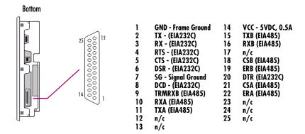
**Note:** Pin 14 is fused with a field-replaceable, 1.0A fast-blow fuse.
