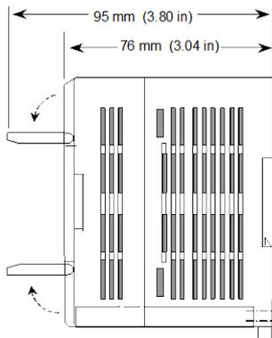
The Micro PLC can be mounted on a wall or panel using screws, or on a DIN rail. The Micro PLC must be mounted on a vertical surface. Do not mount it on a horizontal surface.
