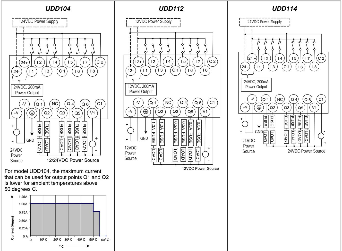
A pull-down resistor, connected between Q# and C1, is required for high frequency Pulse and PWM outputs and for duty cycles in the lower ranges (5% and lower). A 1.5k ohm, 0.5 watt resistor is recommended.
