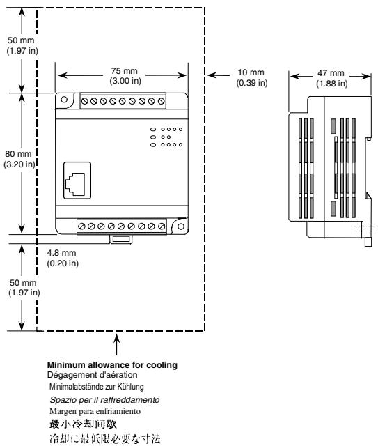
The Nano PLC can be mounted on a wall or panel using screws, or on a DIN rail. The Nano PLC must be mounted on a vertical surface. Do not mount it on a horizontal surface.
