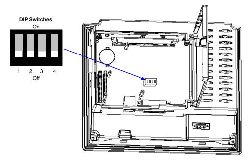
When the switch is set to "OFF", the QuickPanel View operates normally, displaying the startup splash screen. You can skip running the startup applications by tapping the "Don't run StartUp Programs" button on the startup splash screen.
