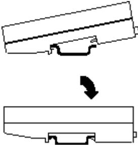
The PROFINET Scanner and connecting carriers must be installed on the same section of 35mm x 7.5mm DIN rail. The rail must have a conductive (unpainted) finish for proper grounding. For best resistance to vibration, the DIN rail should be installed on a panel using screws spaced approximately 6 inches (5.24cm) apart.
