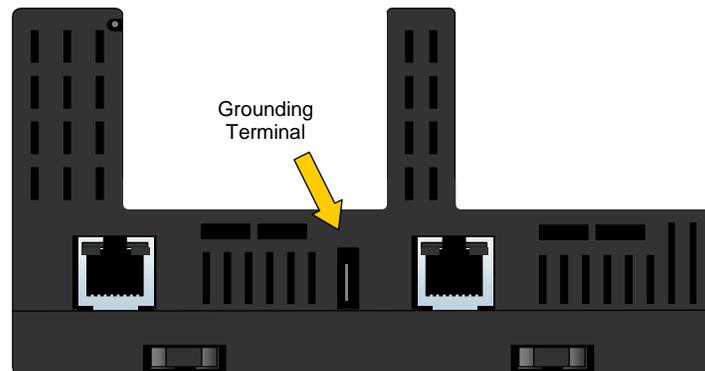
Connect a ring terminal on the other end of the wire to a grounded enclosure. Where the ring terminal contacts a painted enclosure panel, either install a star lock washer between the terminal and the panel to cut through the paint, or scrape the paint away down to clean, bare metal to ensure a good contact.
