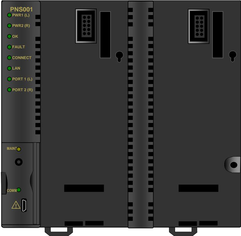
The PROFINET Scanner supports the use of either one or two power supplies. Use of the second power supply is optional. Power supplies mount directly onto the module and latch into place. The illustration above shows the PROFINET Scanner with no power supplies installed.
