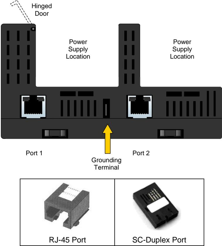
Model IC200PNS001 has two RJ-45 ports, providing 10/100 Mbps copper interfaces. Model IC200PNS002 has two SC-Duplex ports, providing 100Mbps Multi-Mode fiber interfaces. Each Ethernet port automatically senses the type of network and adjusts speed and connection parameters. The PROFINET Scanner requires at least one network be operating at full duplex for a connection to remain established. The PROFINET protocol may be sent and received over either or both of the two external ports.
